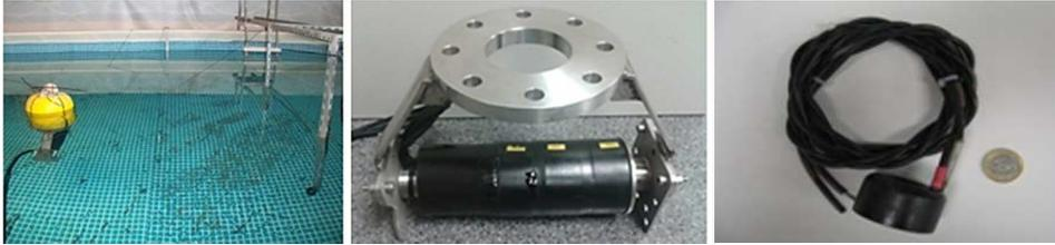
Fig 4.14. Experimental setup (left), emitter (middle) and receiver (right) transducers.
