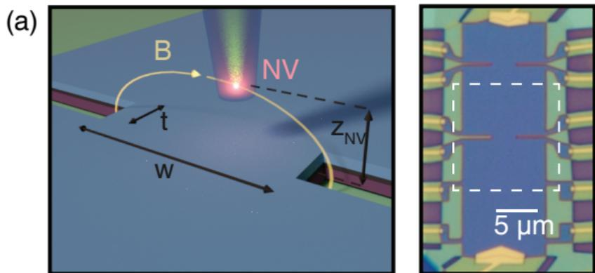
Inverting Biot-Savart we can infer  $\mathbf{J}$  from  $\mathbf{B}$ , with spatial resolution of  $\sim 150\ \text{nm}$ .
