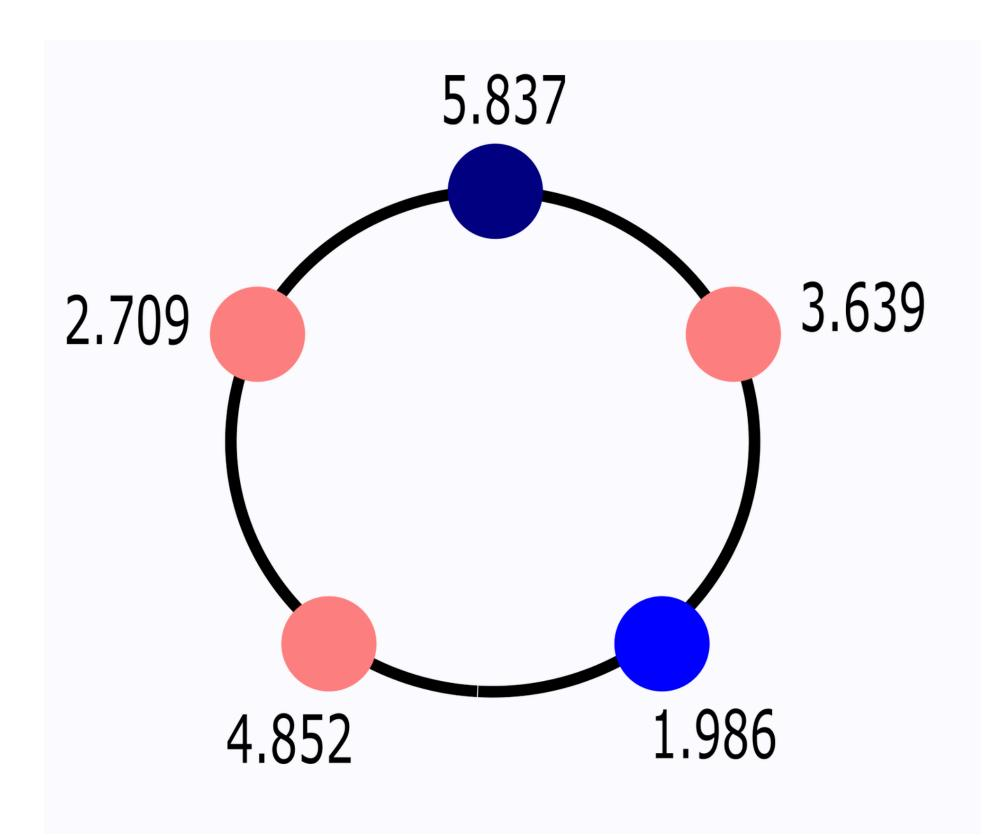
The maximum and minimum phase differences are the positions of the shocks
