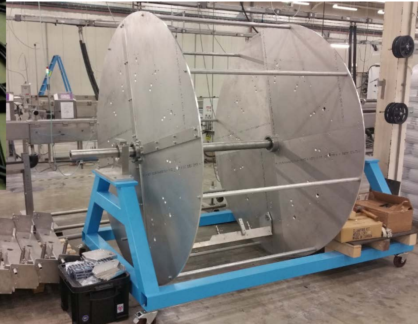
Durham/m2fx constructed planetary cable winding machine
