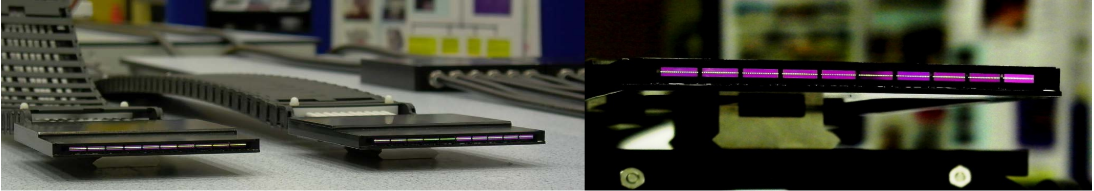
FMOS pseudo slits – non parallel, non-telecentric, low profile, antireflection coated
