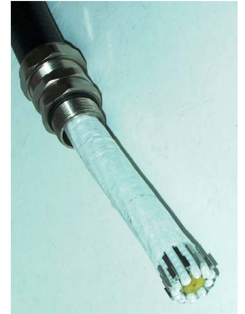
FMOS cable, form replicated in PFS, DESI, and others
