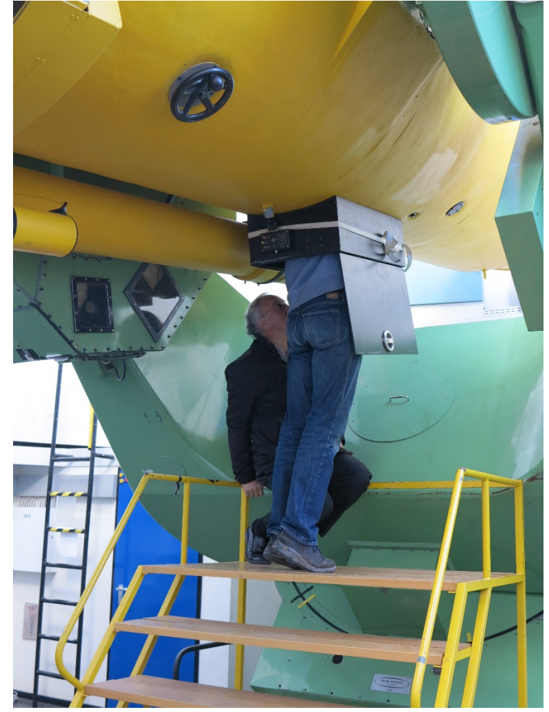
Cassette access port
